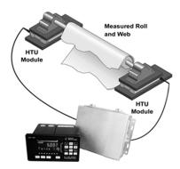
HTU Web Tension Transducers combined with LCt-104 transmitters produce the ultimate in web tension accuracy. HTU transducers supply both horizontal and vertical tension force signals which are resolved by the LCt-104 into the precise resultant tension force and the exact inclination angle. Measurement remains consistent, even if wrap angles change dramatically during the production run. Analog outputs track total force or tension.
