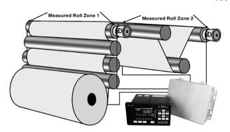
Mode B usually measures two independent tension zones (rolls), each with dead shaft idler roll transducers (4 transducers total). These zones may be two independent points on the same web or any point on two different webs. Mode B analog outputs are roll 1 (transducers 1 & 2) total tension, roll 1 difference, roll two total (transducers 3 & 4), and roll two difference. Mode B also functions with only one, two-transducer tension zone. It is not necessary to use both zones.
